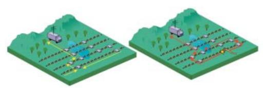
**Figure 2** Multi-path telemetry thanks to multiple transverses. After a break of the receiver line, data are rerouted using another path. Recording can continue before repair of the receiver line.
