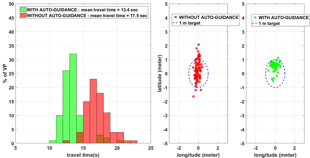
Figure 1: Manual driving vs. Vibrator Auto-Guidance: comparisons of (left) travel time for a 12.5 m distance between VPs, and (right) positioning accuracy.
