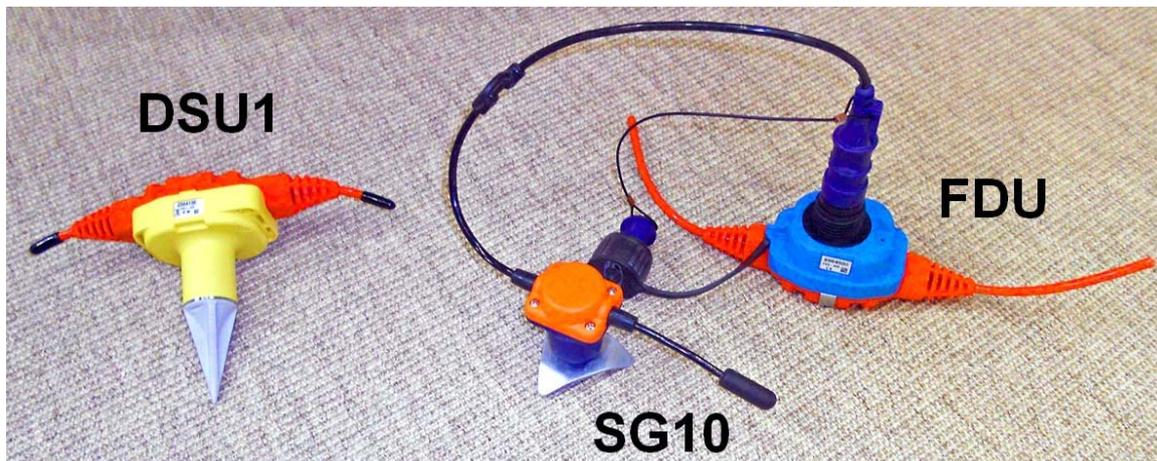
**Figure 1:** Comparison of the Digital Sensor Unit (DSU) with the equivalent vertical geophone (SG10) connected to a digitizer (FDU). DSU1 is more compact and half the weight of the geophone based solution.
