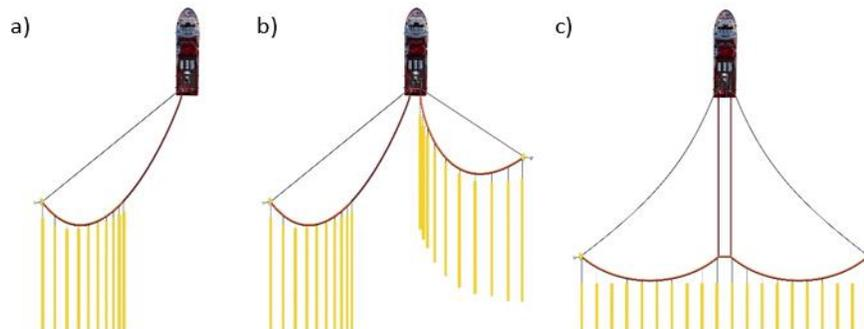
Figure 2: Double deployment process sketch. a) Deployment of the first half, b) Deployment of the second half, c) The full spread as deployed.
