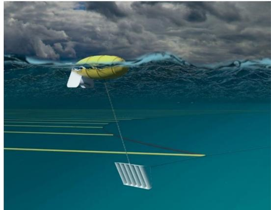
Figure 1: a pelagic-type deflector connected to a surface buoy is used to divert the spread at the desired depth
