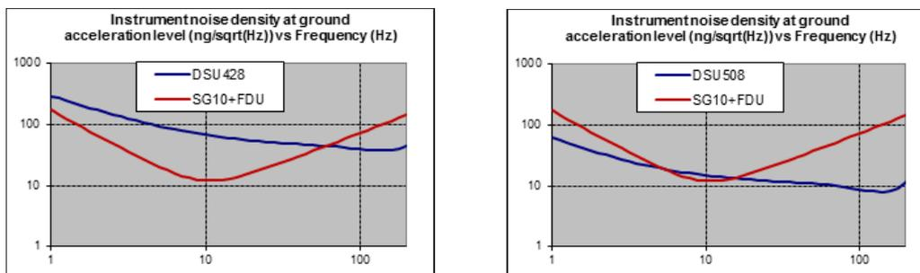
**Figure 2** Comparison in acceleration of the noise floor from different sensors: DSU MEMS 428 (left) & 508 (right) vs. a SG-10 geophone connected to a Field Digital Unit (FDU).
