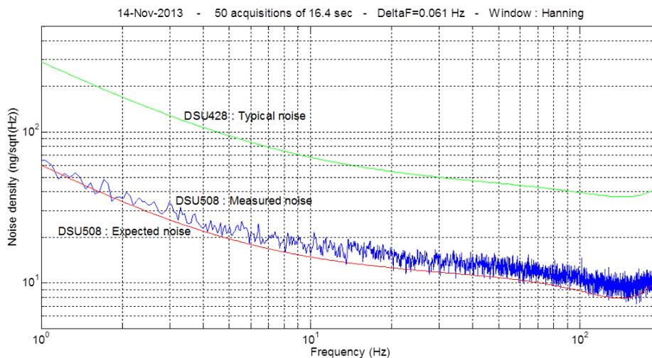
**Figure 4** Noise floor comparison of the vertical MEMS of the DSU-428 & -508: up to -12dB (/4) improvement is noticed in a large frequency range including the lowest frequencies.
