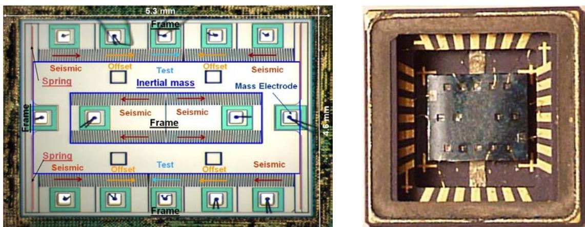
**Figure 1** DSU MEMS architecture as seen by microscope (left) and MEMS in its open ceramic case used to maintain a strong vacuum (right).
