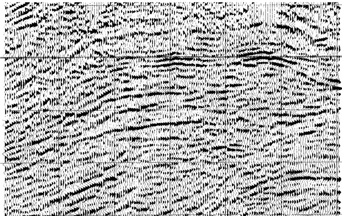
*Figure 1b Simulated conventional 3D data, trace density = 55,296 traces per square mile
