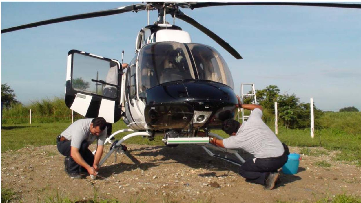
*Figure 3 Data harvesting unit mounted on front of helicopter*
