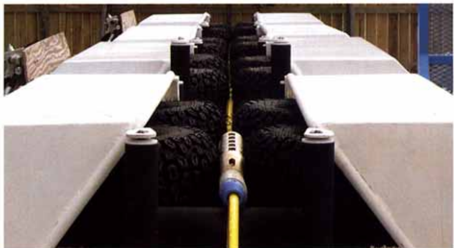
Figure 2. An OBS cable is squitter-tested to replicate cable retrieval forces from maximum depth.
