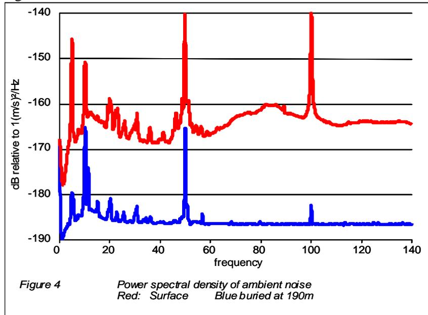
Whithers<sup>(2)</sup> cited by Bormann<sup>(3)</sup> reports a 20 to 40 dB drop in the noise level at a depth of 43m. Figure 4 compares the power spectral densities of the analog component at 190m and of a surface geophone. We found a reduction in seismic noise of 20 to 24 dB at frequencies lower than 30 Hz. Above 30 Hz, electrical noise dominates and the comparison becomes irrelevant.
