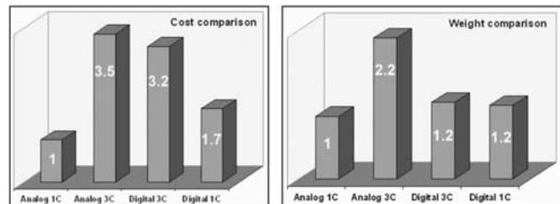
Figure 7: Cost (for CAPEX) and weight (for OPEX) comparison of the four configurations presented in Figure 6. Numbers are relative to the conventional analog 1C configuration (reference = 1).
