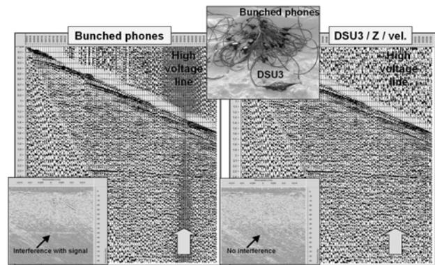
Figure 2: Shot point comparison between digital sensor units (DSU3) and bunched phones (photo). Strong pick up of a high voltage line is due to analog transmission. (Data courtesy of BNGF)
