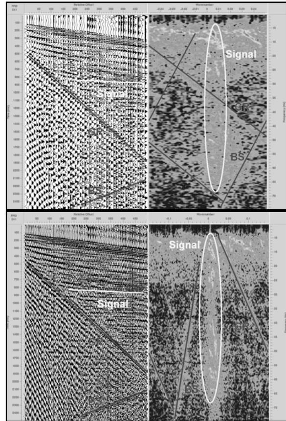
**Figure 4:** Shot point (GR=ground roll, BS= back scattering) with 10 m spacing (top) and 3.3 m spacing (bottom). (Data courtesy of CGG)
