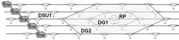
Figure 5: 2D acquisition design that uses single 1C digital sensor units (DSU1) connected along parallel telemetric cables. At a given receiver point (RP) different types of digital groups (DG1, DG2) may be considered to attenuate surface noise.
