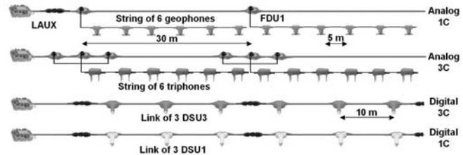
Figure 6: A conventional 6 geophone string receiver point (Analog 1C) is compared with the corresponding Analog 3C receiver point. Assuming one digital sensor may replace two geophones, the corresponding Digital 3C & 1C receiver points are displayed.
