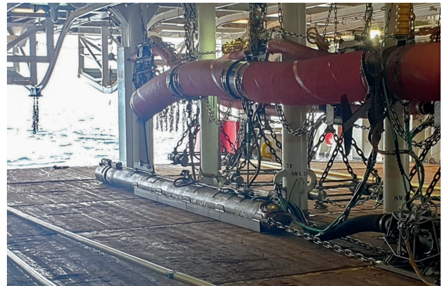
Figure 4 TPS ready to be deployed from the source vessel back deck (full TPS installation video).
