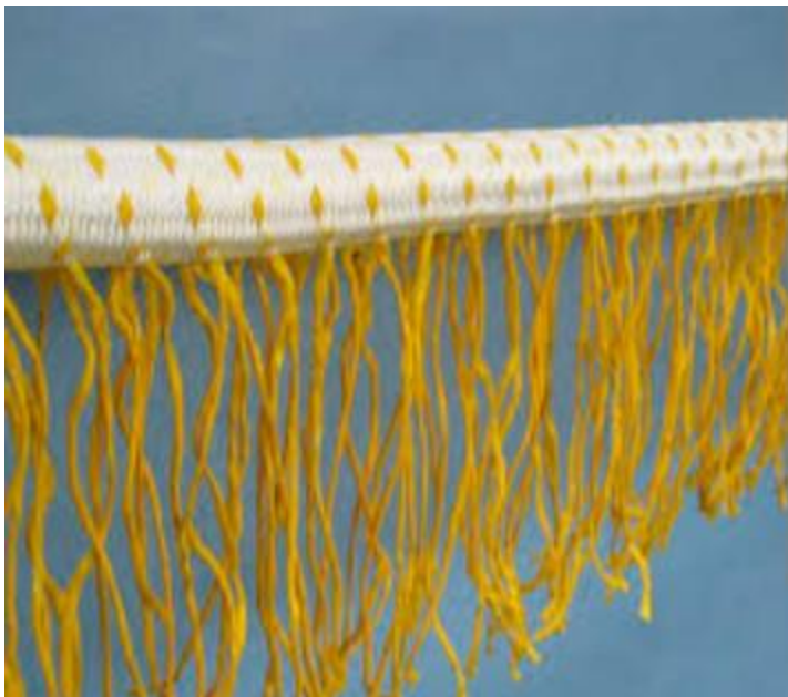
Figure 28. Photo of rope with hairy fairings embedded.
