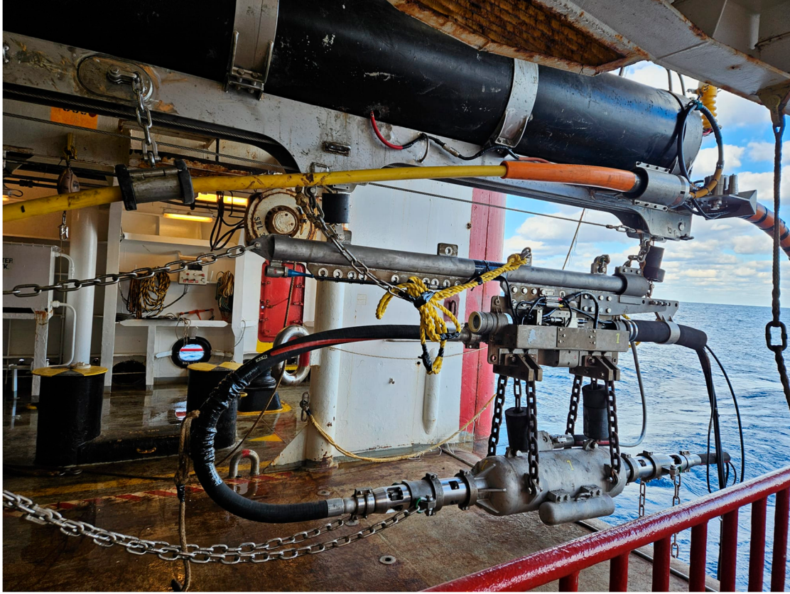
Figure S34. The Gemini Source™ 8,000 in 3 on a dry deck. Photo courtesy of TGS.
